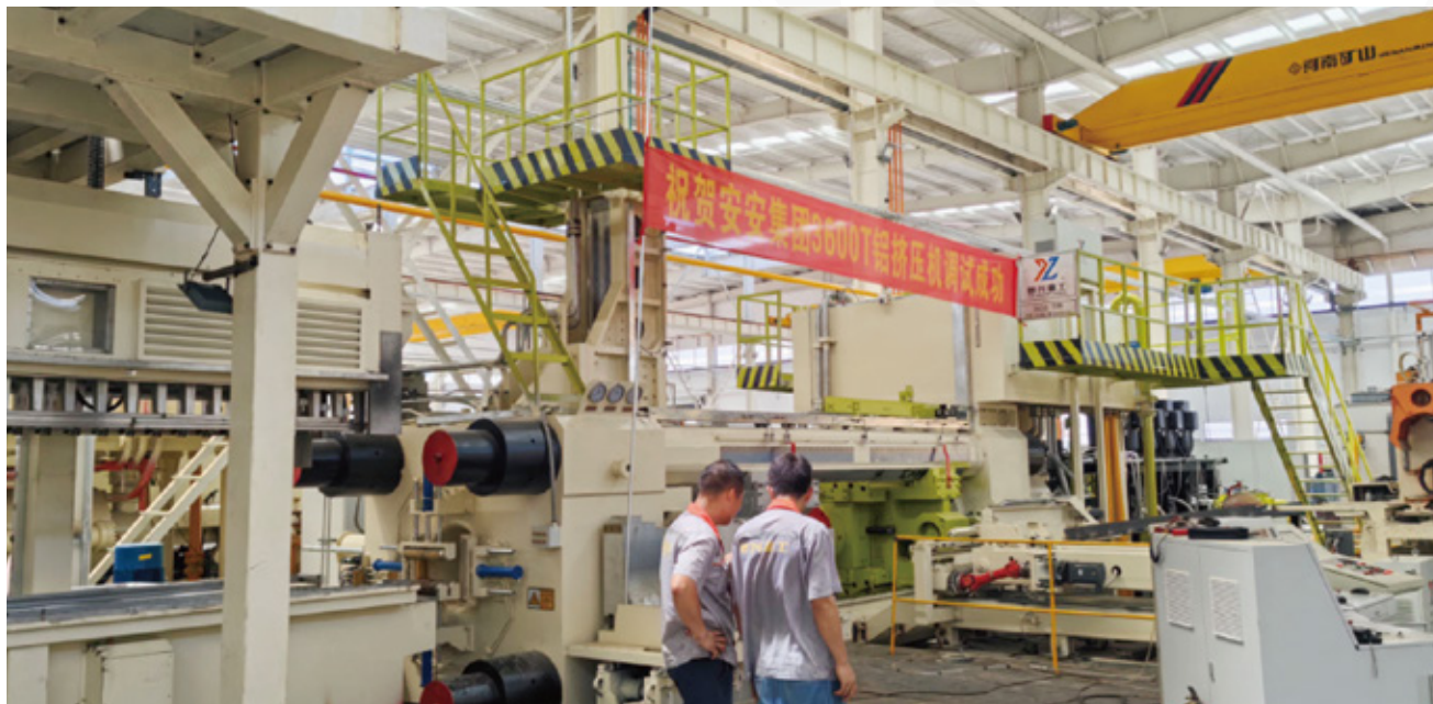
4500MT短行程后上棒挤压机 4500MT SHORT STROKE REAR UPPER ROD EXTRUSION PRESS
