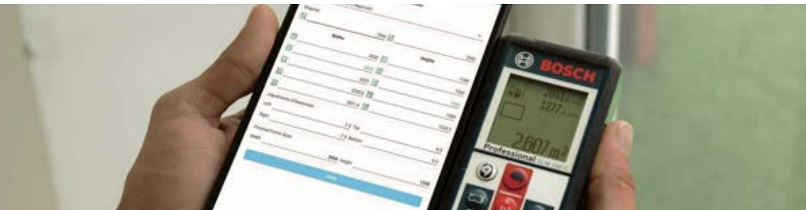
Automatic measurements via bluetooth using Bosch laser device
