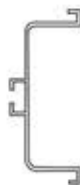
TCH-8744 Aluminium Gola Profile (G- Shape) Specification • Finish : Aluminium / Black • Size : 3mtr.
