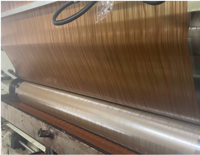
Technical Details - 20-micron film | 1630mm x 1000 meter
