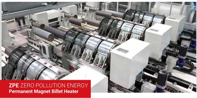
Presezzi Extrusion has developed the revolutionary ZPE (Zero Pollution Energy) magnetic billet heater to meet stringent environmental standards and lead the aluminum extrusion industry towards a cleaner and more efficient future.
