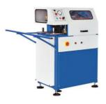
•Input Power: 1.5Kw •Power Supply: 380V/50Hz •Working Pressure: 0.5 ~ 0.8MPa •Motor Rotary Speed: 2800r/min •Air Consumption: 100L/min •Profile Width: 20 - 120 mm •Profile Height: 20 - 120 mm •Drawing Groove Width: 3mm •Drawing Groove Depth: 0.3mm •Overall Dimension: 1650 x 1300 x 1450mm •Weight About: 270 kg
