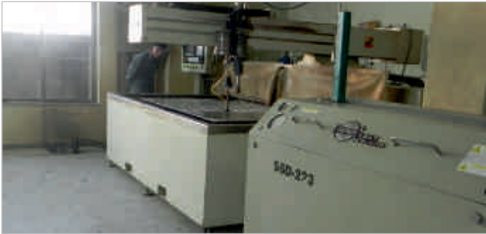
WATER JET CUTTING MACHINES
