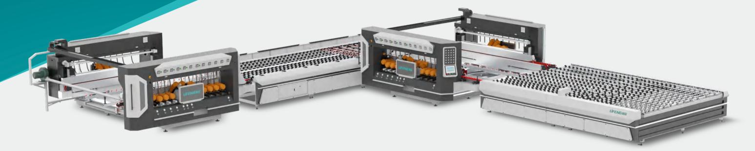
Adopt precise and high efficient automatic detection table to realize automatic adjustment of any size; High speed opening and closing at 25m/min; High-speed edging up to 20m/min. All grinding wheels are automatically compensated, reducing the level of manual operation. Equipped with an intelligent operating system, the master control and scheduling are integrated, and the operation of the entire line can be easily controlled.
