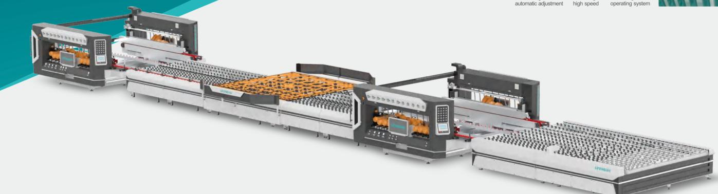
Adopt precise and high efficient automatic detection table to realize automatic adjustment of any size; High speed opening and closing at 25m/min; High-speed edging up to 20m/min; Automatic compensation for polishing grinding wheel; Equipped with intelligent operating system integrated control and scheduling, easy control the operation of the whole line.
