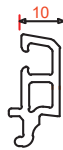
EWSPL - LF - 1008 Sliding Double Glazing Bead (EWSPL - LF - 1008-WG) Sliding Double Glazing Bead with Gasket
