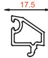
EWSPL - LF - 4005 Sliding Sleek Single Glazing Bead (EWSPL - LF - 4005-WG) Sliding Sleek Single Glazing Bead with Gasket
