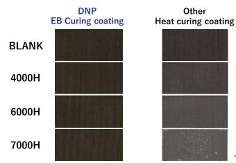
No changeColour fading, BubbleTest Method : ISO4892-2Xenon-Arc light exposure
