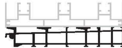
Water Drainage Track Section Number : V-3523 Weight (kg/mt) : 2.049
