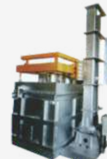
Fixed degas-unit 固定式在线除气箱
