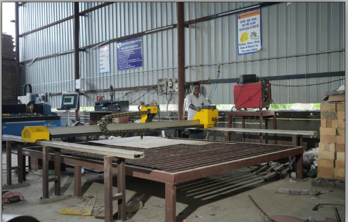
PLASMA CUTTING UPTO 40 MM SHEET
