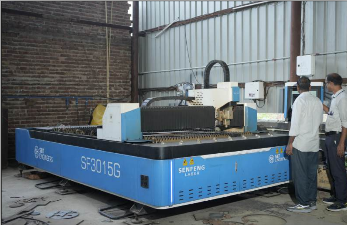
LASER CUTTING FOR HIGH PRECISION CUTTING UPTO 20 MM SHEET
