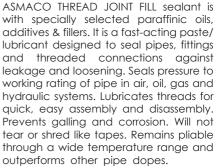
• Easy to use • Non drip formula • Effective up to 5000 psi • Good heat resistance • Temperature range –65°F to +300°F (-54°C to +204°C)
