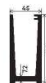
Continuous Railing Bottom Section Number : V-10003 Weight (kg/12') : 14.875
