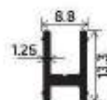
"H" Type Adapter Section Number : V-2534 Weight (kg/mt) : 0.121
