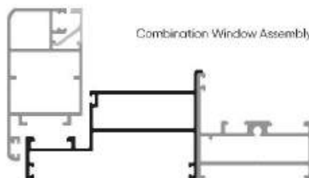
Combination Frame Section Number : V-5112 Weight (kg/mt) : 0.859
