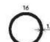
Grill Fitting Tube Cover Section Number : V-1002 Weight (kg/mt) : 0.164
